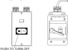
Figure 11. Power ON/OFF Switch (OFF)
